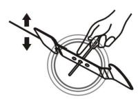
The blade is made of hardened steel. To get a clean job, sharpen the blade frequently, about every 25 hours of use. Make sure the blade is always well balanced. Insert a small iron pin (2 or 3 mm in diameter) into the hole in the middle of the blade: it must remain horizontal. If the blade does not stay horizontal, balance it by sharpening it further on the side where it is leaning.
