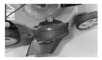
You must fit the mulching adapter in order to use the side ejector. Hook in the side ejector adapter.
