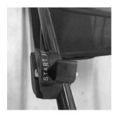
For a hot start, move the lever to the position marked: RUN
